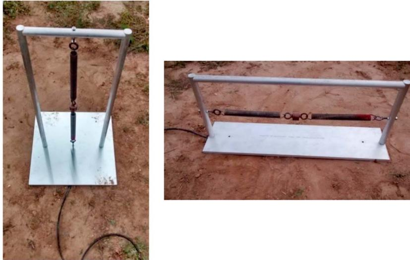
**Figure 9.** (left) Vertical mass-spring apparatus to exert controlled normal pressure on the ground, and (right) horizontal mass-spring apparatus to exert controlled shear stress on the ground.
