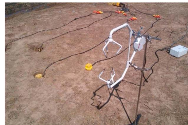
**Figure 5.** Experimental setup for the geophones and the anemometer.
